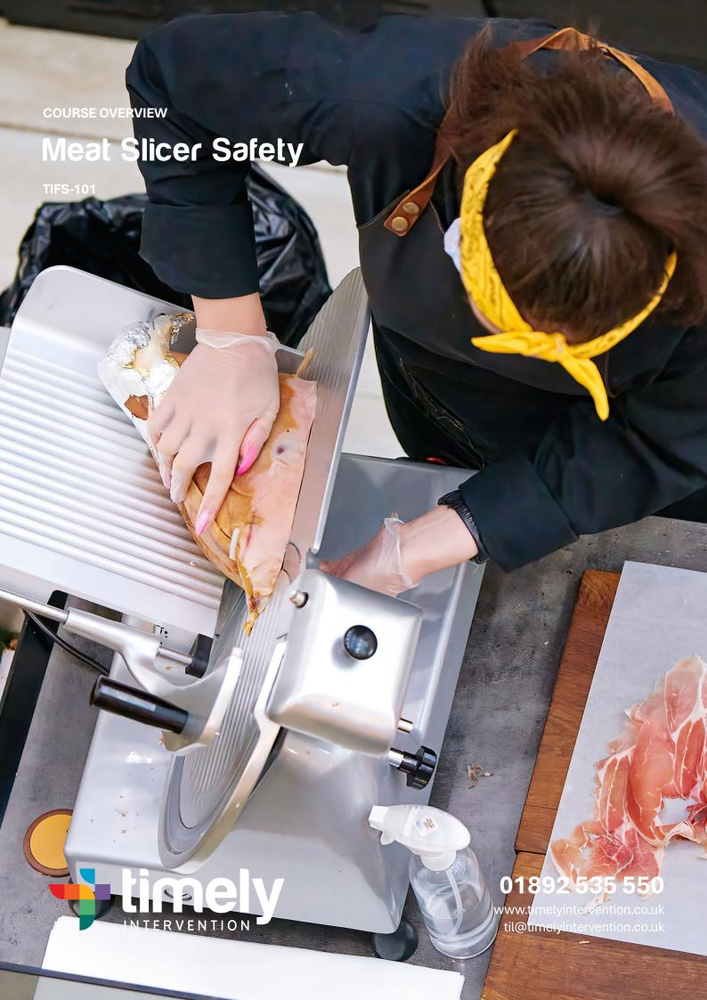
Meat slicers are vital tools in delis, restaurants, supermarkets, and grocery stores, offering fast and precise cuts of meat. However, their high-speed rotating blades pose a constant safety risk, even when the machine is not actively slicing. Injuries from meat slicers can range from minor cuts to severe lacerations and even finger amputations.
